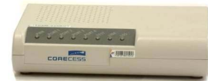
Corecess 3802TW - 1 port SuperPON, 20Km - 1 port 10/100Base-TX & 1 port 10/100/1000Base-T
